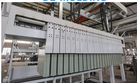
5. ROBOTIC ARM GRIPPING GYPSUM BLOCK
