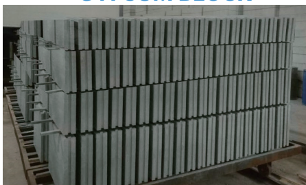
8. COMPLETED DEHUMIDIFY FOLLOW BY PACKAGING
